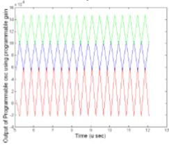
**Fig.7** Output with Programmable Amplitude with CCCII current gain on-chip programming. Output (Red) corresponds to CCCII gain=1.0769, blue corresponds to gain=1.1886 and green corresponds to gain=1.2138.
