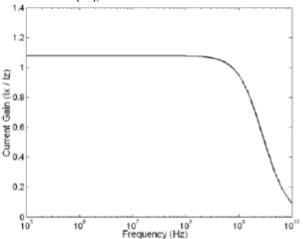
Fig.2 Frequency response of Current gain of CMOS CCCII design with basic circuit configuration
