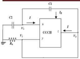
**Fig. 5** Simplified circuit schematics of the CCCII based Oscillator. In our proposed design we employ programmable CCCII aforementioned to generate programmable oscillations.
